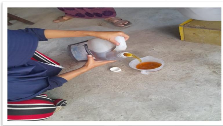
Gambar 2. Pencampuran air, mijel dan NaOH
