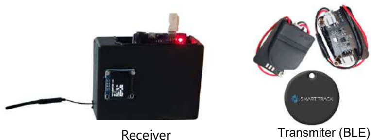
Receiver Transmitter (BLE) Gambar.9 Desain Rangkaian SMART Track
