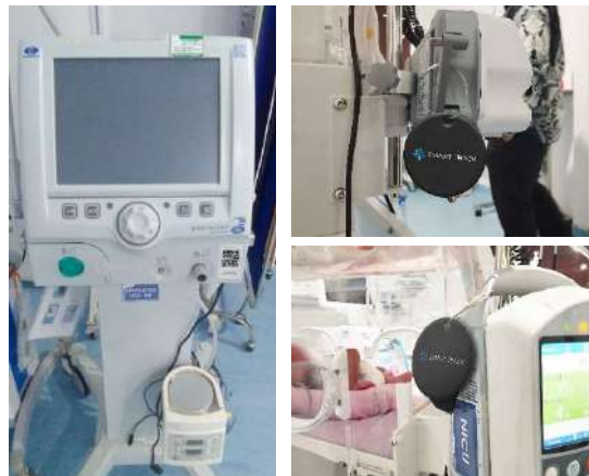
Gambar.11 Instalasi Rangkaian di beberapa Alkes (Ventilator, Infusion Pump, Syringe Pump)
